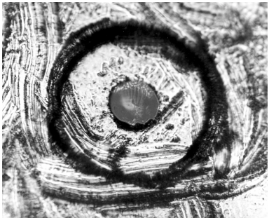
Figure 2-6. Damage from improper cleaning.
